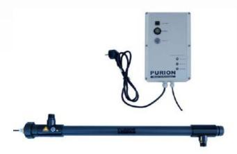
UV Plant PURION 2500 36W is equipped with PVC-U reactor. PURION 2500 36W can be used to disinfect drinking water up to a flow rate of 2.500 l/h and a transmission of at least 90% per cm.
