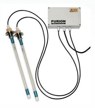
The UV Set DUAL consists of two quartz-made protective tube which are closed at one end while the other one is placed into stainless steel flanges, two UV radiators, one switching box with electronic cut-in unit and the connecting cables.
